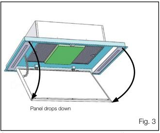
**Step 1d:** After swinging open the panel/panels on any of the cassettes, disconnect the lighting by depressing the tabs on the connection plug and pulling the cable.
